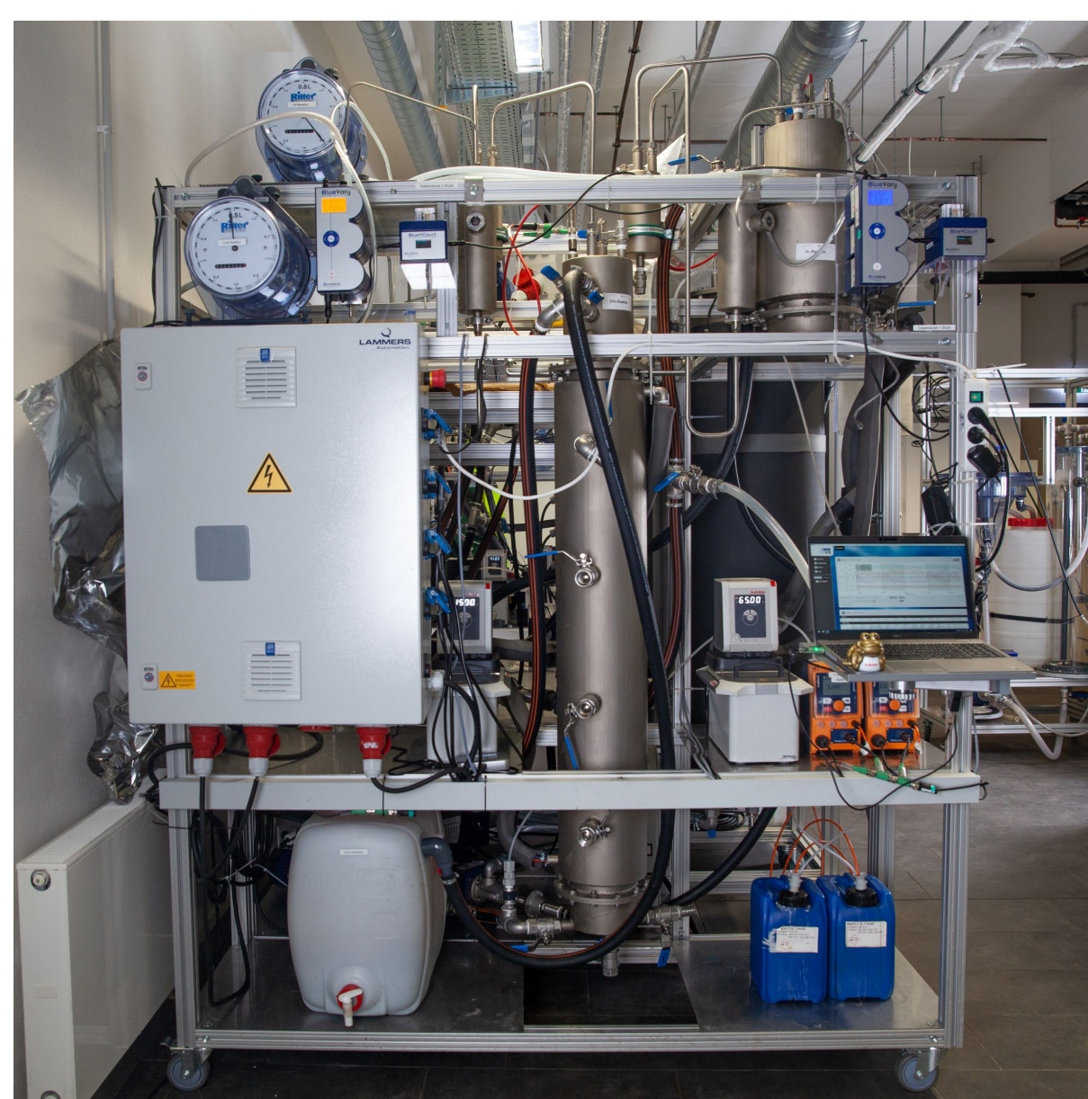
Figure 2: Two-stage test plant for biological production of hydrogen via dark fermentation.
