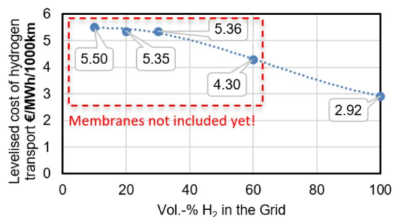
Figure 4. First set of results for levelized hydrogen transport costs via existing pipeline transmission system (retrofitted) at different admixture levels
